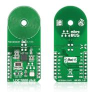
LDC1000 click<sup>™</sup> carries the world's first inductance-to-digital converter IC, along with a detachable sensor (an LC tank comprising a 36-turn PCB coil and a 100pF 1% NPO capacitor). The board can be used for short range measurements of the position, motion or composition of conductive targets. LDC1000 click<sup>™</sup> communicates with the target board through mikroBUS<sup>™</sup> SPI (CS, SCK, MISO, MOSI) and INT lines. The board is designed to use either a 3.3V or a 5V power supply.
